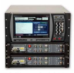
**IFF-7300S-50** - This system configuration includes the test system with two each IFF-45TS's. Optional external UUT power supply is available to add IFF and TACAN UUT test capability.
